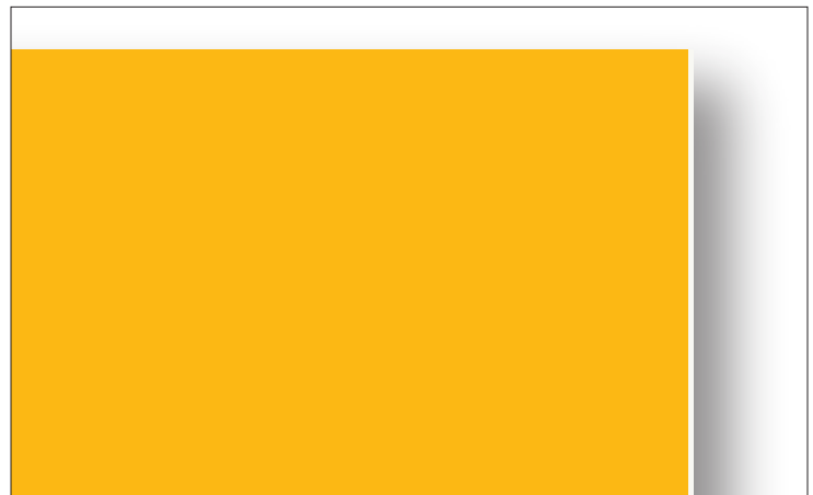
The illustration above represents what can happen when the bleed on the right is short. Notice the paper showing through on the right edge where the bleed is short.
